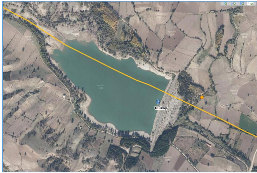
Fig. 3: The location of Ulukoy dam on active fault map (yellow line represents the main segment of NAFZ).
